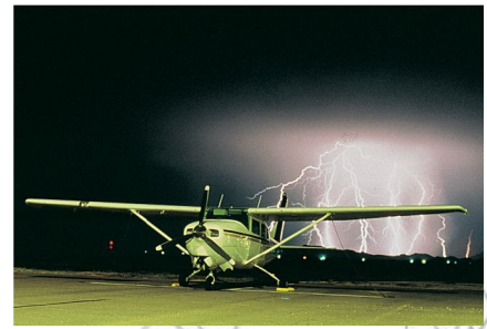
Figure 4.48 Inside a hollow conductor, the electric field is zero even when there is a very strong electric field outside the conductor. The metal body of this plane forms a good shield against atmospheric electric fields, so that the occupants are quite safe from atmospheric electrical discharges (lightning!). Hollow conducting shields like this are called Faraday cages. They are effective because of the two types of electric charge – there is no equivalent of the Faraday cage for gravitational fields.
