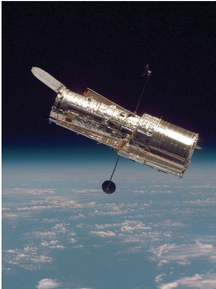
Figure 6.23 The Hubble Space Telescope makes use of gyroscopes to help with moving the telescope to point at the position in the sky correctly
