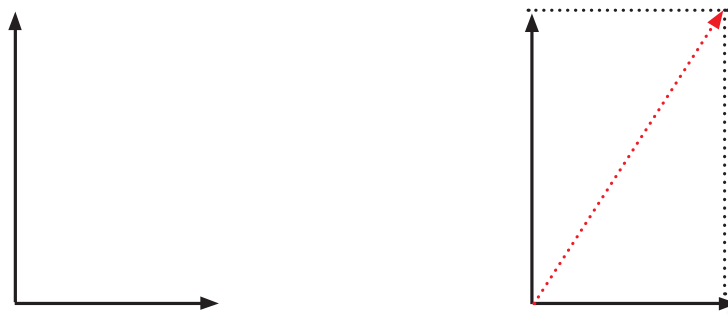
Figure 2.18 Two perpendicular coplanar vectors
