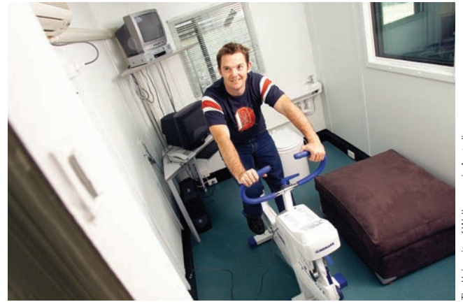
Figure 2.14 Whole-room calorimeter with direct and indirect calorimetry capability.
