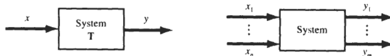
Fig. System with single (a) or multiple input and output signals (b).
