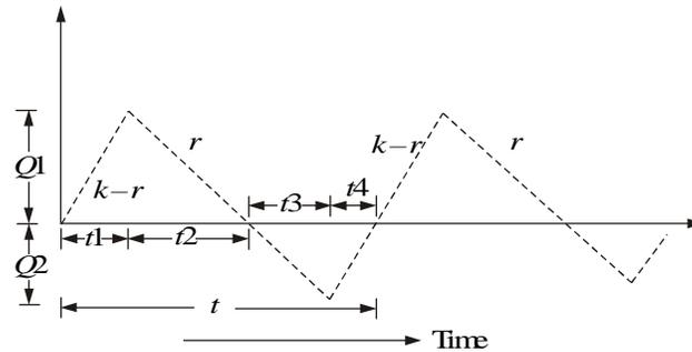
Fig. 12.5 Manufacturing model of inventory with shortages.
