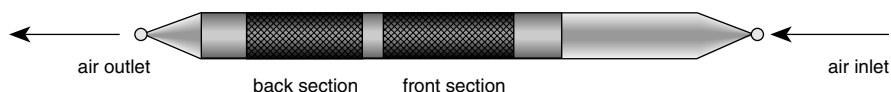
Figure 9.7 Glass tube containing solid adsorbent for collecting samples of airborne gases and vapors.
