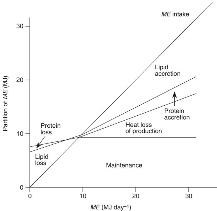
Fig. 11.2. Partition of energy in a pig of 60 kg live weight for different rates of daily intake of ME.
