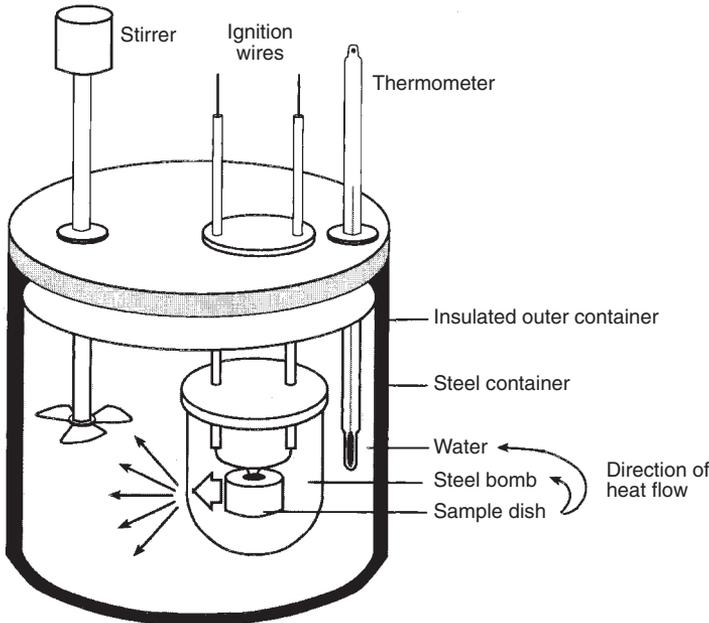
Fig. 11.1. Bomb calorimeter.
