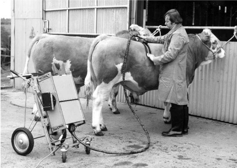
**Fig. 14.6.** Photograph of Scanogram in use on live bull (by courtesy of the Meat and Livestock Commission).
