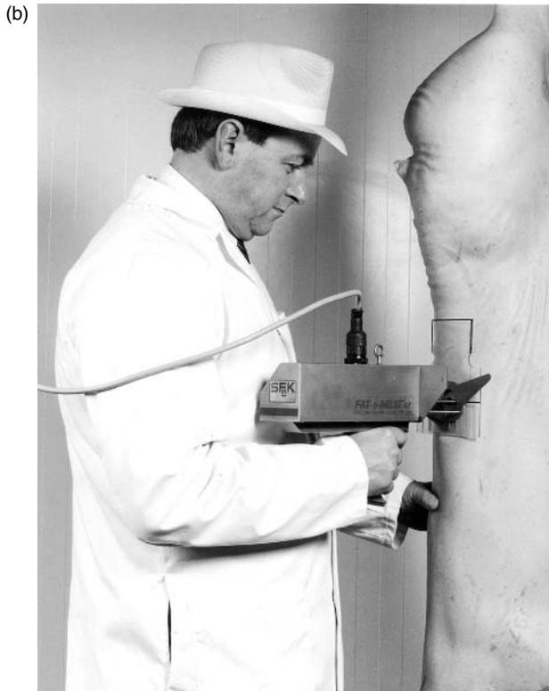
**Fig. 14.7.** Fat-O-Meater automatic probe in use on carcasses on pig slaughter line (a) and in close-up on an individual pig (b). Reproduced by kind permission of the Meat and Livestock Commission.
