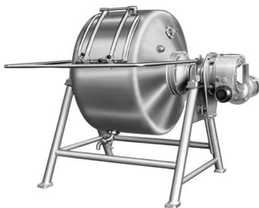
Figure 11.7. Batch butter churn (APV Unit Systems, Denmark).
