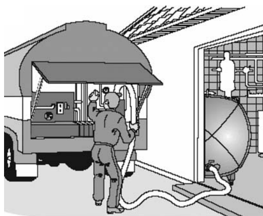
Figure 7.2. Collection of milk on the farm. The tanker is pumping milk from the farm bulk milk tank for transport to the dairy factory. Reproduced with permission from Tetra Pak.
