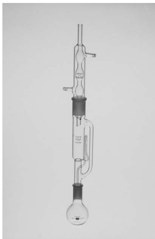
Figure 23.4. Picture of a Soxhlet apparatus for fat determinations. (Picture courtesy of Kimble Chase.)
