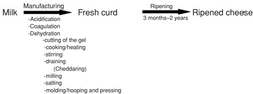
Figure 12.1. General description of steps involved in the cheese manufacture. (Modified from Singh et al., 2003a.)
