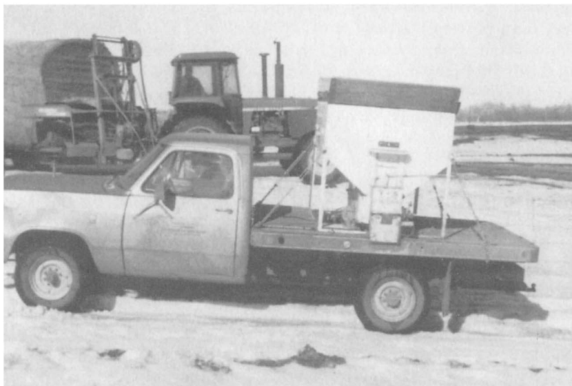
FIGURE 3.7 Equipment developed by the Fort Keogh Livestock and Range Research Laboratory, Miles City, MT, to improve uniformity of supplemental intake by range cattle by spaced placement on the ground includes: (1) a cube drop unit mounted on a pickup, and (2) a mobile unit (shown in background) for transporting large bales or small stacks of alfalfa hay and slicing into segments for dispensing.
